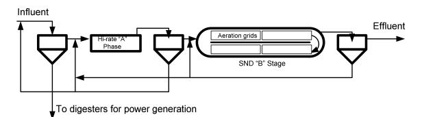
Figure 3 Diagram of Strass, Austria plant with high rate first stage and channel aeration system for SND
